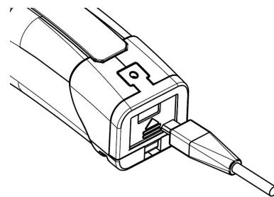
The recharging battery cover has a hole through which a USB power plug (not included) can be inserted into the USB socket on the rechargeable battery inside.
