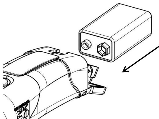
Remove the screw securing the Battery Cover to the case. Install the batteries according to the positive and negative terminals ( + , - ) in the battery slot.
